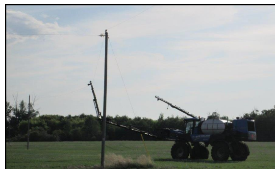
Sprayer contacting a power line.
